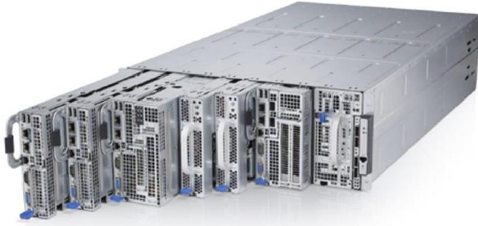
Cada servidor do tipo PowerEdge C8220X "Zeus" node contains two Xeon E5-2680 processors and 32 GB of system memory
